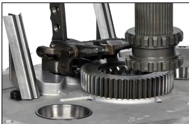
Step 11: Remove the mainshaft and 4th-5th collar.
