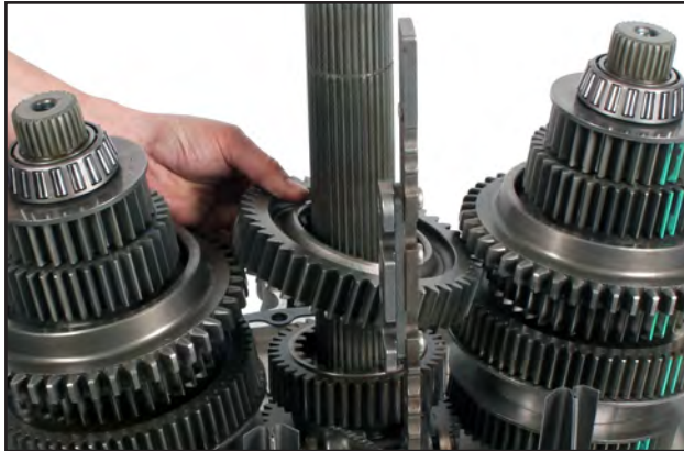
Step 7: Remove the 3rd speed gear
