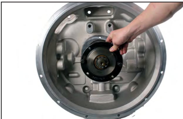
Step 17: To remove the input shaft and front bearing retainer, remove the four bearing retaining bolts. Pull the shaft from the housing. It may be helpful to place 2 bolts in the threaded bearing retainer holes to remove the front bearing retainer. Tap the input shaft out of the clutch housing.
