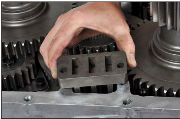
Step 9: Install the rear shift fork support bar. Torque the 2 bolts to 34-41 lb-ft.
