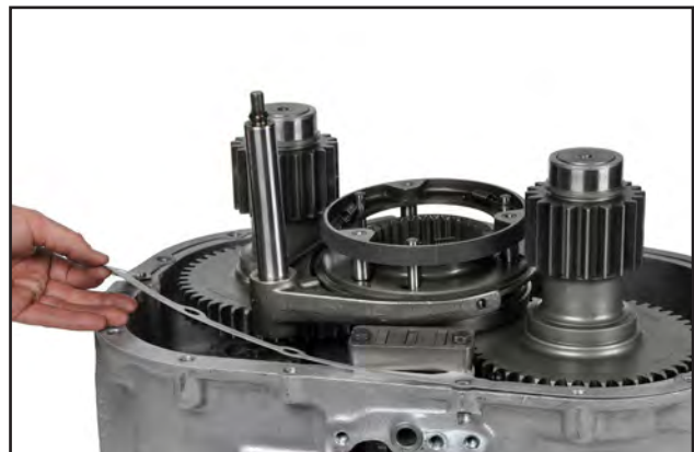
Step 12: Install new gasket.
