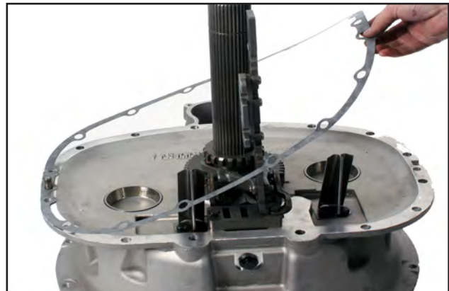
Step 10: Remove the gasket.
