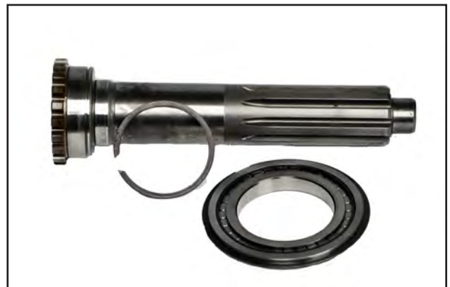
Step 18: To disassemble the input shaft assembly, remove the snap ring. Press the bearing off the shaft.
