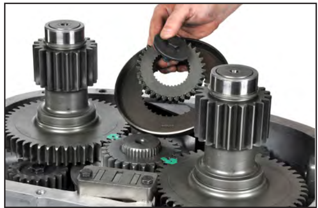
Step 10: Install the high range clutch gear and the synchronizer cup. Secure with washer and bolt. Torque to 78-98 lb-ft.
