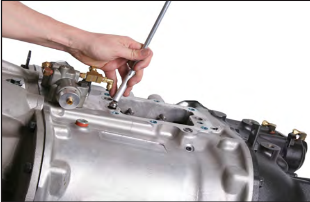
Step 7: Remove the 3 poppet balls located under the springs.
