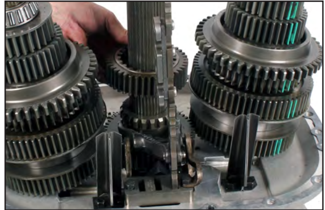
Step 8: Remove the 4th speed gear (5th gear if working on an overdrive transmission).
