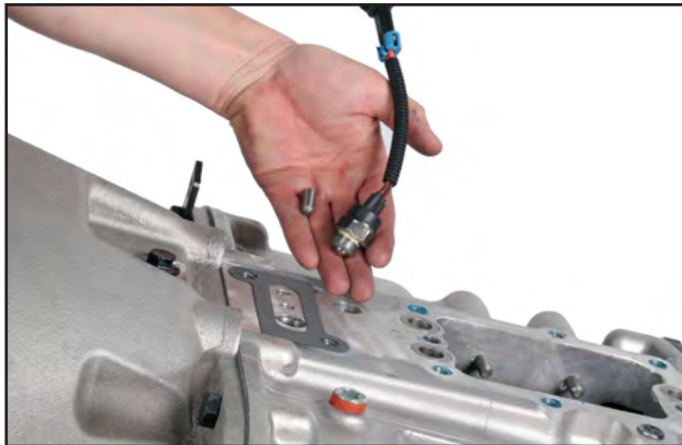
Step 9: Remove range control valve gasket. Remove the backup light switch and pin
