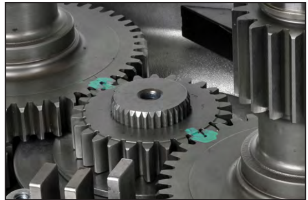
Step 8: Be sure to align the timing marks as the high range gear is installed.
