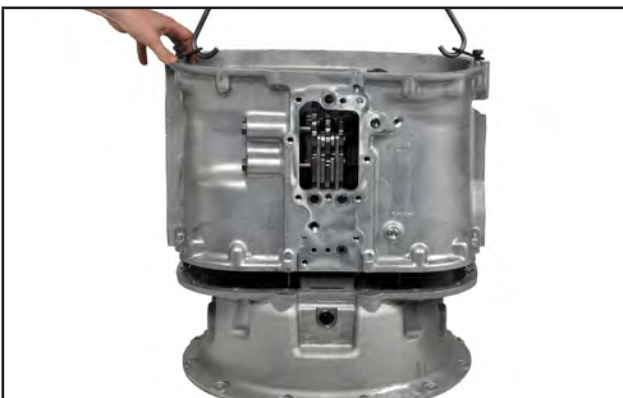
Step 17: With the aid of a hoist, lower the main case into position. Install the case bolts and torque them to 78-98 lb-ft.
