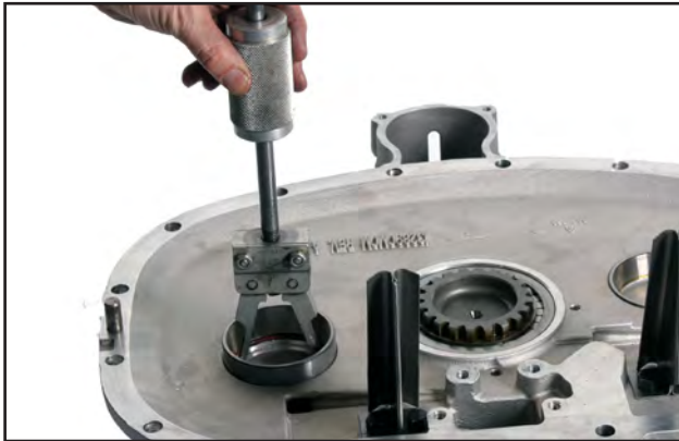
Step 15: Remove the countershaft front bearing cups as shown.
