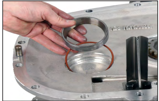
Step 16: Inspect O-rings in clutch housing.
