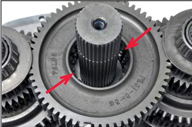
Step 13. Note the equal spacing around the mainshaft.
