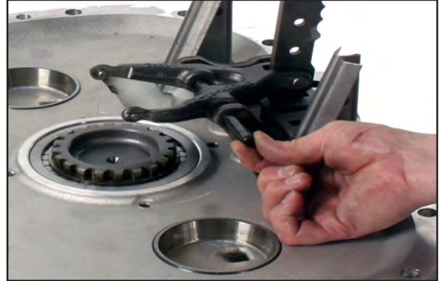
Step 14: To remove the 4th-5th speed shift fork, remove the snap ring. Push the pin through the bracket. Lift the fork from the unit. Remove the 4th-5th shift fork support brackets.
