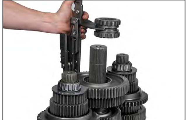
Step 14. Install the 1st-reverse shift fork and collar. Double check timing by shifting each sliding collar into its mating, or respective, gear.
