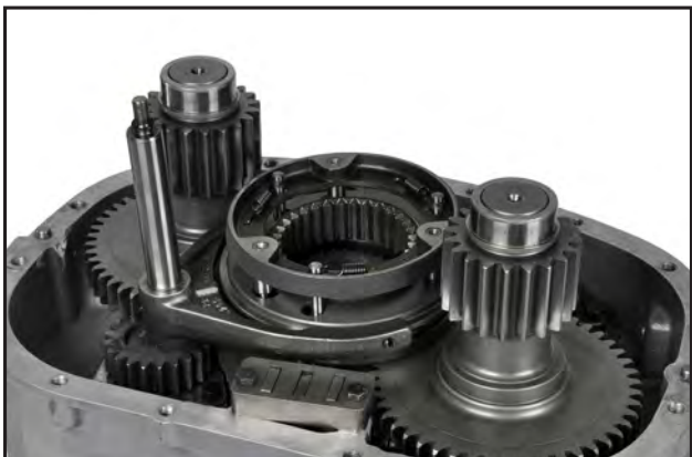
Step 11: Install the range synchronizer and range fork with the synchronizer springs facing toward the output yoke or flange.
