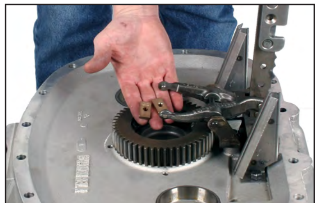
Step 12: If the 4th-5th speed shift fork shoes are worn, replace them. It is not necessary to remove the fork to replace the fork shoes.
