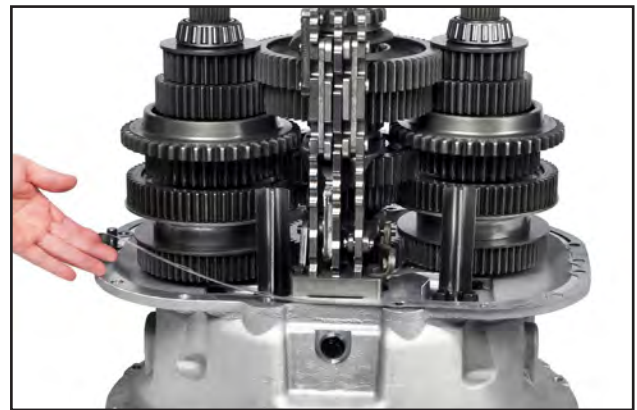
Step 16: Install new gasket.
