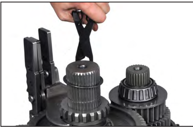
Step 15: Install mainshaft snap ring.
