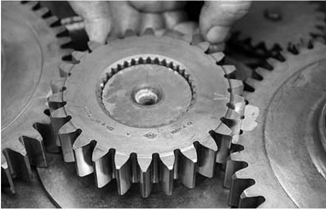
17. Lift high range gear from the case.
