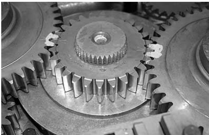
9. Now install the high range drive gear. Align the timing marks.
