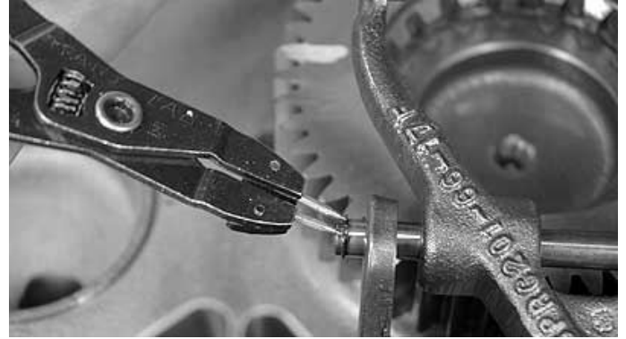
14. To remove 4th-5th speed shift fork, remove the snap ring. Push the pin through the bracket. Lift the fork from the unit.
