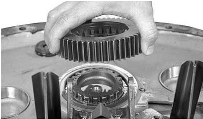
15. The 5th speed (direct) gear or 4th speed (overdrive) gear is removed next. The oil troughs can remain with the case.
