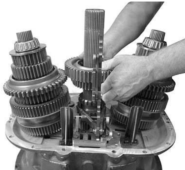
8. Slide 3rd gear (clutching teeth up) and 4th gear (clutch teeth down) speed gears over mainshaft.
