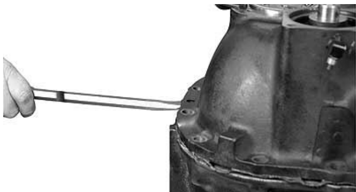
12. Remove the range case bolts. Using pry bars in the milled slots will make case removal easier.
