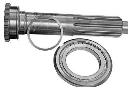
19. To disassemble the input shaft assembly, remove the snap ring. Press the bearing off the shaft. Make sure you wear safety glasses to protect your eyes.
