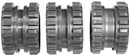
17. Notice that the fork slot the 4th-5th speed shift collar is wider than the fork slot on the other collars in an overdrive transmission. In a direct transmission all collars will be the same.
