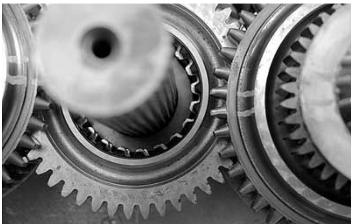
9. Tilt countershafts inward to engage 3rd-4th speed gears. Make sure there is equal spacing around the mainshaft and internal teeth.
