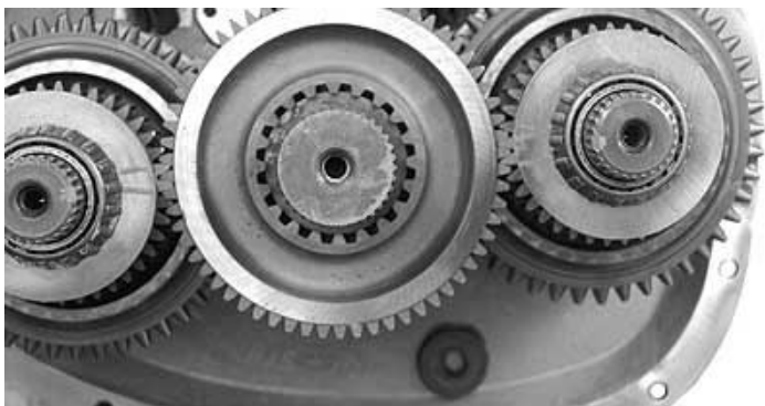
11. Slide 2nd speed gear onto mating countershaft gears. Make sure to maintain equal spacing around mainshaft. Clutching teeth facing down.
