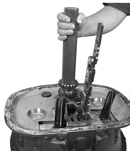
12. Remove mainshaft and 4th-5th clutch collar.
