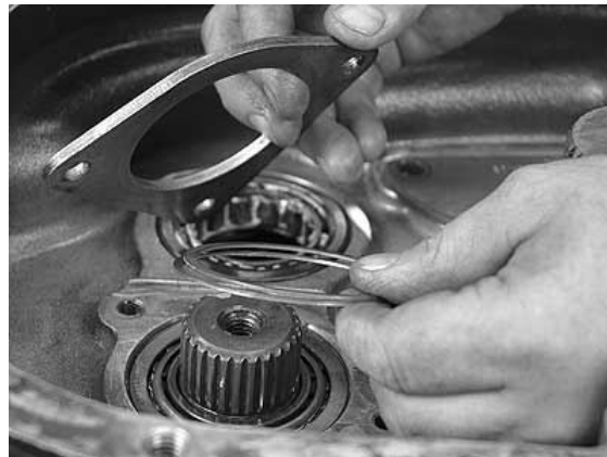
23. Next remove the right countershaft rear bearing retainer plates and shims.
