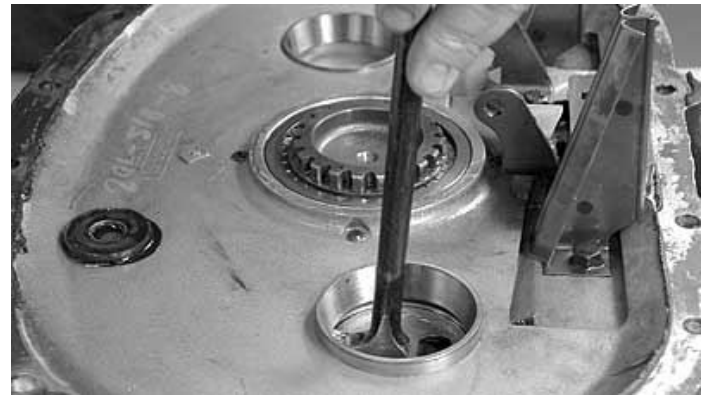
16. Remove countershaft front bearing cups as shown.
