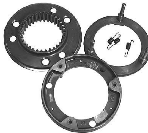
! 15. Be aware that separating the synchronizer will suddenly release the springs. Always wear safety glasses to protect your eyes when servicing transmissions. Synchronizer replacement parts may be purchased separately.
