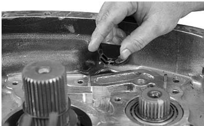
22. Remove the left countershaft retaining bolts and retaining plates. Also remove the oil passage bypass valve.
