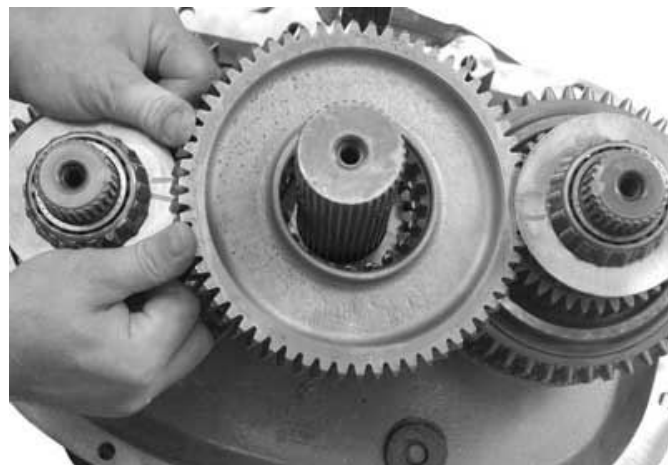
12. Install 1st speed gear as shown. Clutching teeth facing up.
