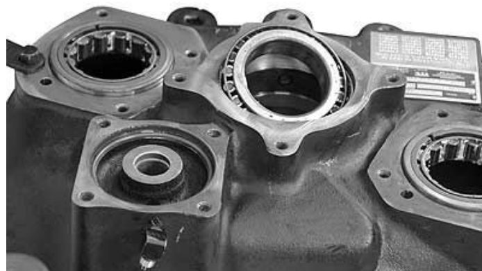
25. Remove the output shaft bearings from the case. Wearing A safety glasses, press the inner bearing from the shaft.
