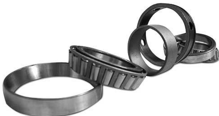
! 26. These bearings and spacers are a matched set. If it is necessary to replace any of the components, the whole set must be replaced. Replace them as a set to help ensure proper end play.
