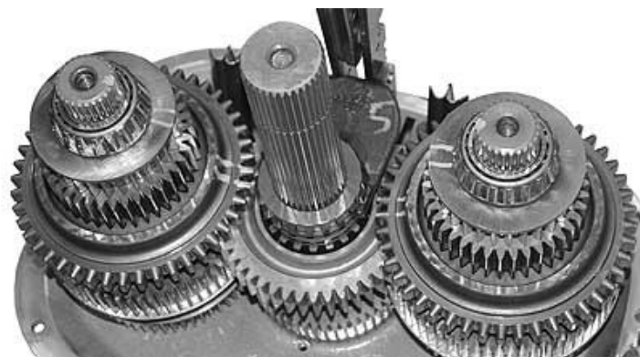
10. Install 2nd-3rd clutch collar and fork.
