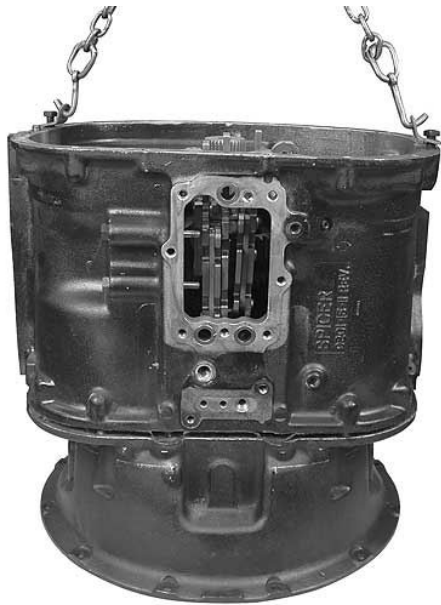
15. Apply Loctite® 515 or the equivalent to the clean housing face. The using a hoist, lower the main case into position. Install the case bolts and torque them to 78-98 ft. lbs.
