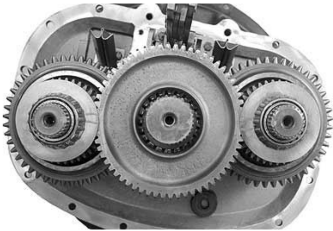
13. Note the equal spacing around mainshaft.
