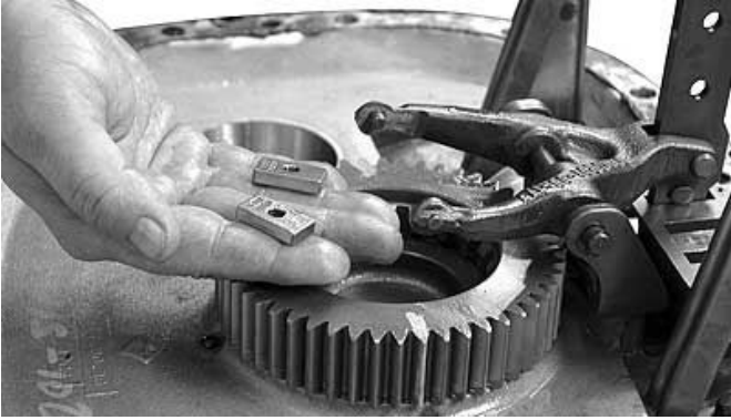
13. If the 4th-5th speed shift fork shoes are worn, replace them. It is not necessary to remove the fork to replace the fork shoes.
