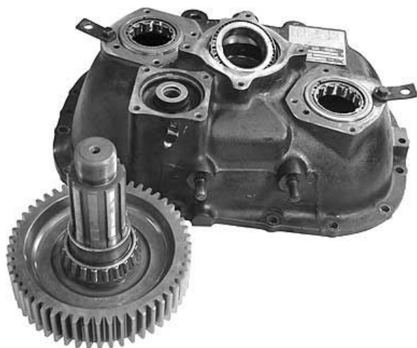
24. Remove the output shaft from the case.
