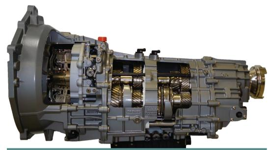
Tremec's TR-9007 is a 7-speed DCT with a torque capacity of 900Nm, a suitable fit for high-performance applications
