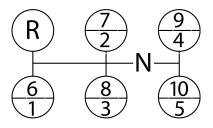
The simple 10-speed shift pattern lets drivers concentrate on driving for greater safety.
