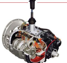
PRO-SHIFT<sup>™</sup> 10-Speed transmissions are designed for over-the-road and city applications. TTC offers many configurations of the PRO-SHIFT 10-Speed, including a complete line of direct drive and overdrive configurations. For weight sensitive or bulk hauling applications, consider our OPTI-LITE<sup>™</sup> and OPTI-LITE II<sup>™</sup> options. They reduce transmission weight and allow you to haul more payload.
