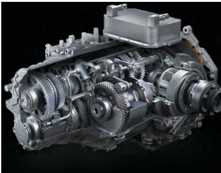
A look inside the new Tremec 8-speed DCT. The transaxle's input shaft is positioned as on a racecar, below half-shaft height to facilitate mounting the engine lower in the car.
