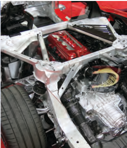
C8 Corvette gear ratio chart and DCT installation (at right). The TR 9080 will skip ratios, as long as both even and odd gears participate in the downshift, i.e., 7th to 4th, 6th to 3rd, or 5th to 2nd.
