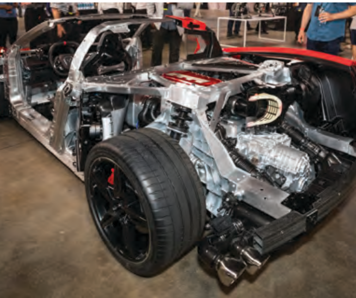
Uncloaked view of GM's new mixed-materials flagship shows extensively-webbed castings serving multiple structural roles, along with various aluminum sheet and extrusions. Note exhaust routing, fan location ahead of rear wheels, airbox design, and GM-Tenneco electronically-tunable exhaust outlets.
