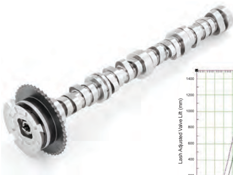
A new, more aggressive camshaft design and a phaser with greater authority conspire to increase the LT2's volumetric efficiency.
