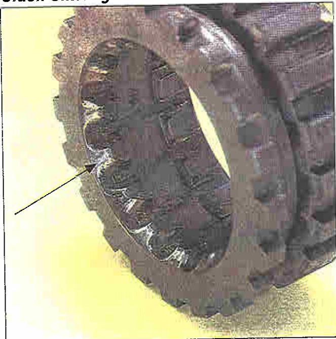
Worn clutching teeth indicate a clash shifting condition.
