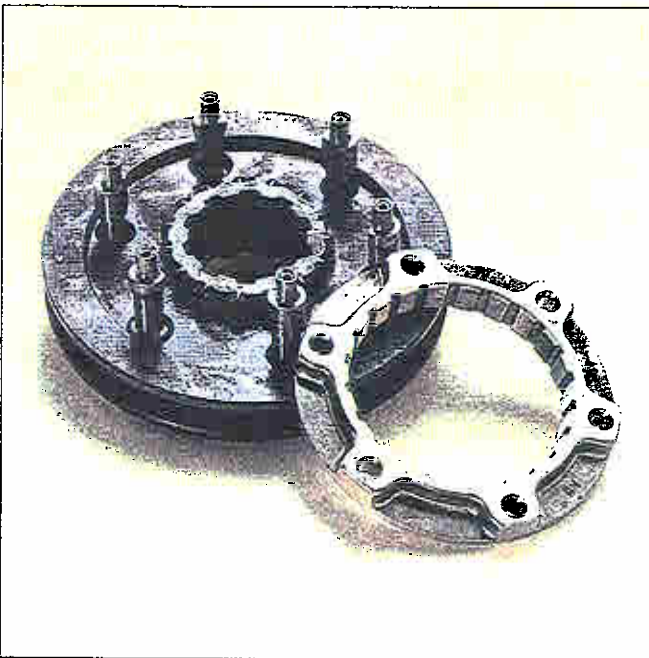
Figure 18—Vibration can cause the brass ring to separate from the rest of the synchronizer.
