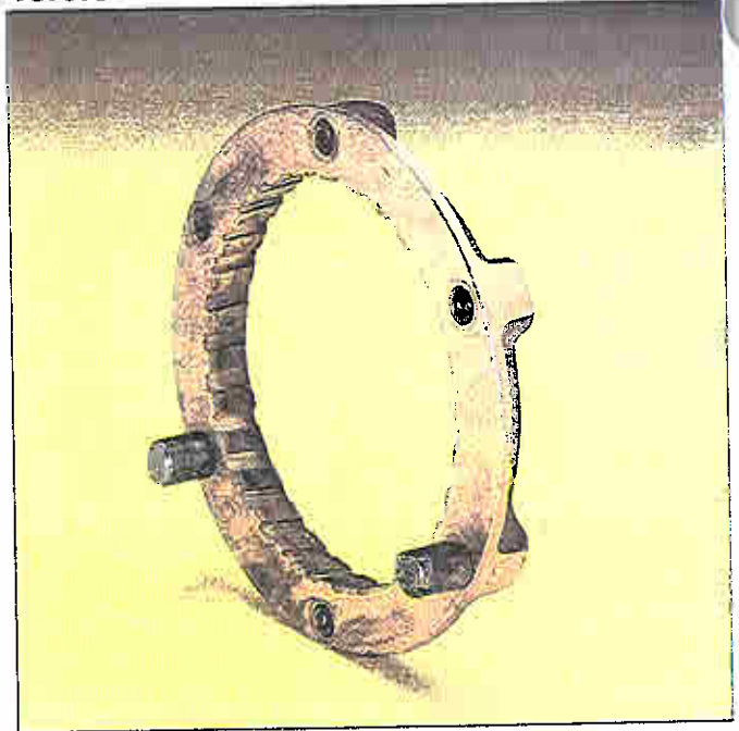
Vibration can cause the brass ring to separate from the rest of the synchronizer. Sheared synchronizer pins are also a sign of vibration.
