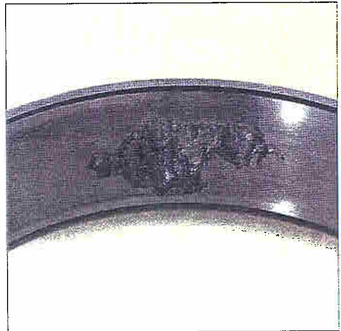
Figure 10—Offset spalling is caused by misalignment.
