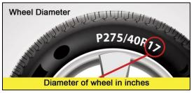
**Wheel Diameter** is the size of the wheel measured from one end to the other. It tells the size of the wheel that the tire is intended to fit. A size 275/40R17 tire is made for a wheel with a 17 inch diameter.
