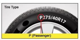
**Tire Type.** The letter "P" at the beginning of the tire size indicates that the tire is a P-Metric tire, referring to tires made to certain standards within the United States, intended for passenger vehicles. The use of P-Metric sizes began in the late 1970s and they are the most frequently used type of tire size today.
