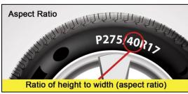
**Aspect Ratio** is the ratio of the height of the tire's cross-section to its width. For example, in a P275/40R17 tire, the 40 means that the height is equal to 40% of the tire's width. The bigger the aspect ratio, the bigger the tire's sidewall will be.
