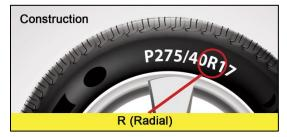
**Construction.** The letter "R" in a tire size stands for Radial, which means the layers run radially across the tire.
