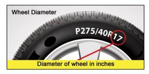
**Wheel Diameter** is the size of the wheel measured from one end to the other. It tells the size of the wheel that the tire is intended to fit. A size 275/40R17 tire is made for a wheel with a 17 inch diameter.
