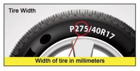
**Tire Width** is the measurement from the widest point of its outer sidewall to the widest point of its inner sidewall when mounted and measured on a specified width wheel. It is measured in millimeters. In this example, the width of the tire is 275 mm.
