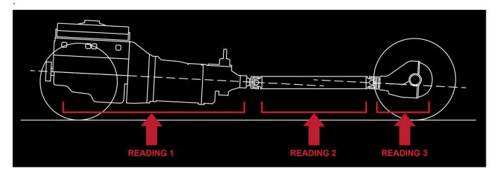
*Important:* All readings must be taken from the same side of the vehicle, Orientation from the driver side is recommended.
